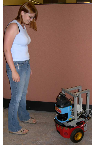
Fig. 3. Robot engaging user by aiming camera and microphone at target
