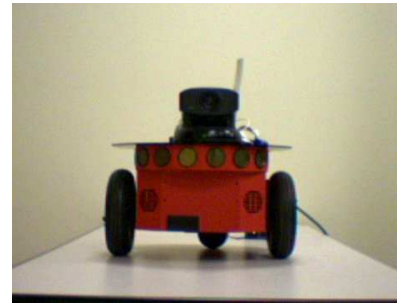
Fig. 3. The ActivMedia Pioneer 2 DX robot used in the experiments, as seen in the remote robot setting. The motions of the PTZ camera provide feedback that supplements the audio.
