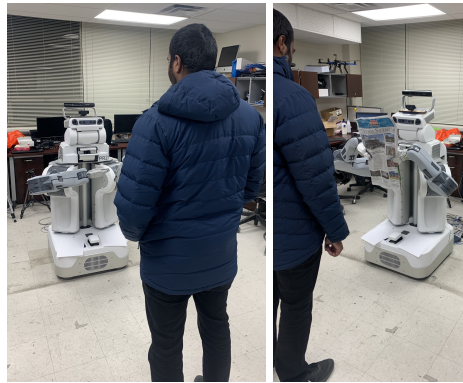
Figure 3.8: PR2 robot displaying two different gaze behaviors. left: PR2 robot making eye contact with the approaching participant; right: PR2 robot distracted reading newspaper when participant approaches the robot.
