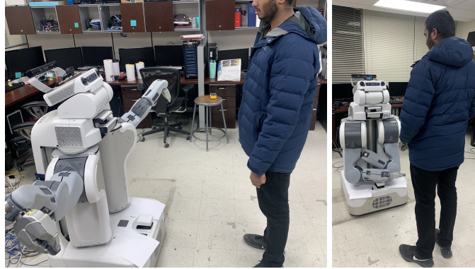
Figure 3.7: PR2 robot demonstrating two different arm positions. left: PR2 robot's arms extended when participant approaches the robot; right: PR2 robot's arms tucked in at the time when participant approaches the robot.
