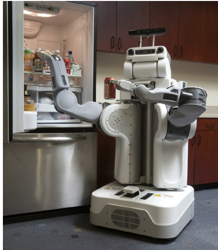
Figure 3.2: PR2 robot with height set at 133cm
