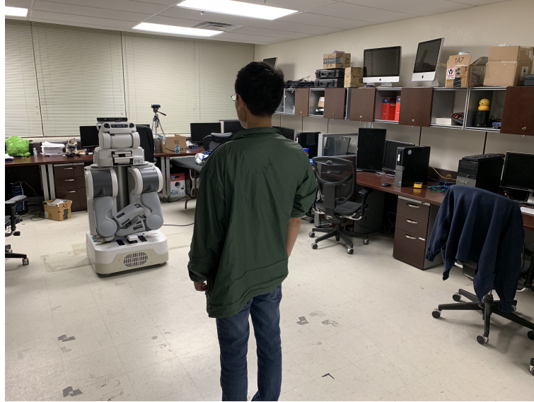
Figure 3.5: Task 2 being performed with the PR2 robot in which the robot approached the social zone
