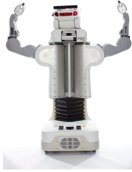
Fig. 2: PR2 robot with height set as 164.5cm referred as PR2 Tall
