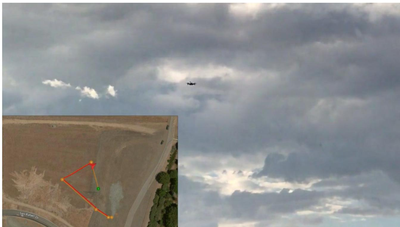
**FIGURE 9.** Waypoints set for the experiment on the physical drone in real time. The attack was discovered after the UAV navigated after waypoint 4 and Return-to-Launch (RTL) was enabled. The drone was able to travel back the originally deployed position. Video link: <https://www.youtube.com/watch?v=TXwQiGoNsjw&feature=youtu.be>
