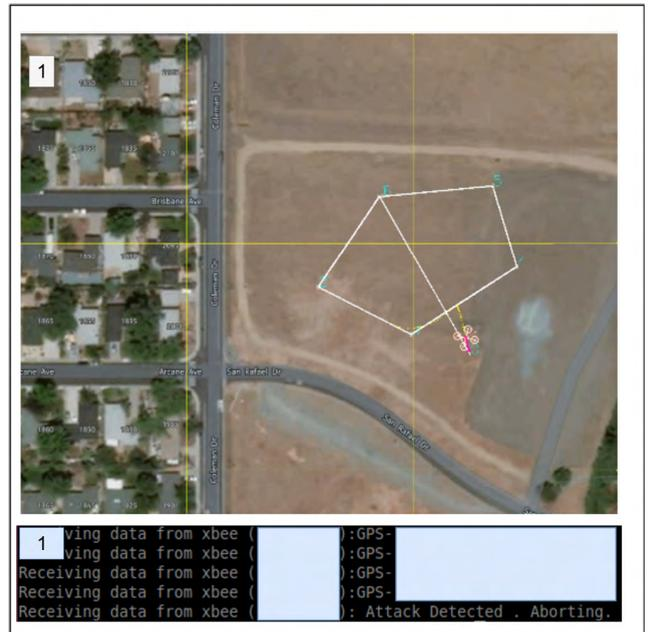
**FIGURE 5.** Waypoints set for the experiment in the first configuration. The attack was discovered after the UAV navigated from waypoint 3 and Return-to-Launch (RTL) was enabled. The drone was able to travel back the originally deployed position.
