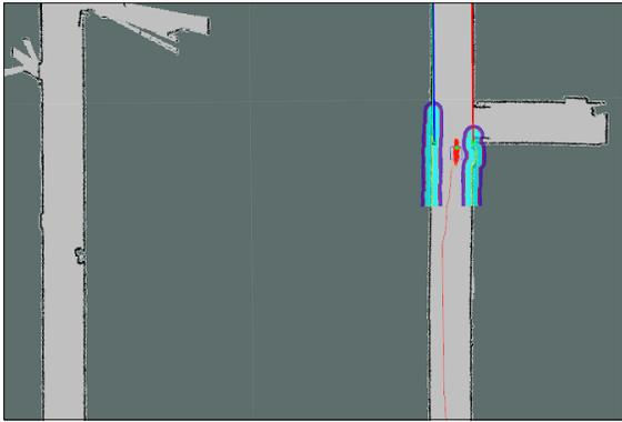
Fig. 2. Rviz screen capture showing robot navigation in the simulated environment and the detected hallways represented by line markers.
