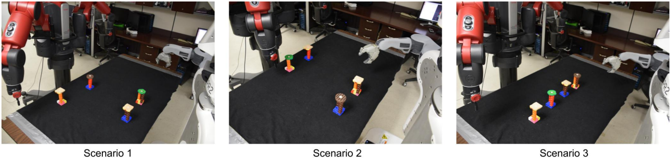
Fig. 3. A view of each of the three setups for the simple behavior experiments. Each scenario has different locations for the objects as well as different initial positions for the right gripper of each robot.
