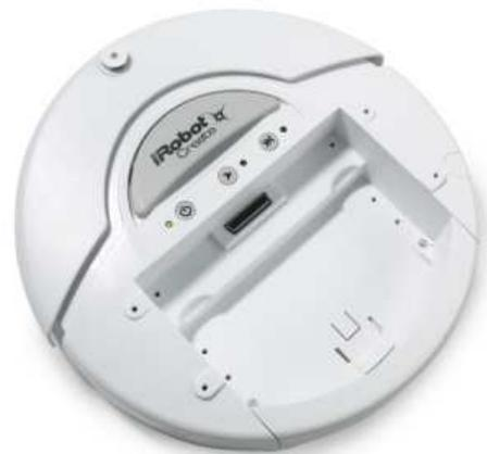
Figure 2: iRobot Create programmable robot.
