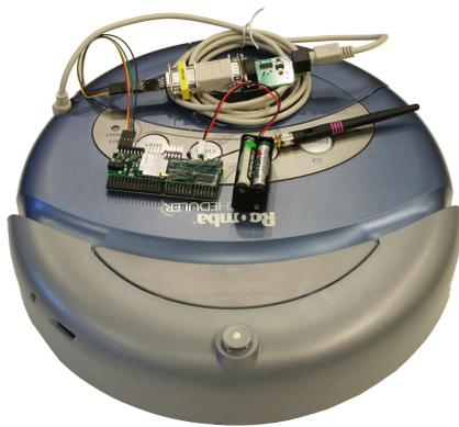
Figure 3: iRobot Roomba vacuum cleaner robot attached to a Gumstix computer.
