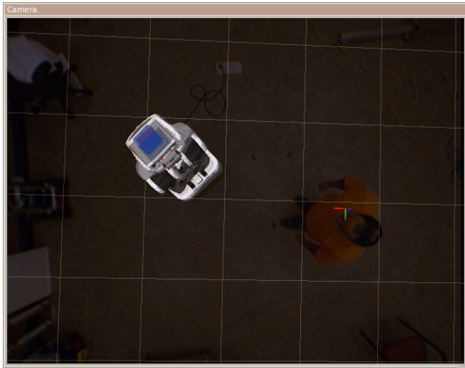
Fig. 1. A view from the overhead camera with a pose overlay of the robot and axes showing the detected position of the social partner.
