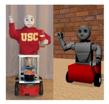
Figure 1: An example of an HRI testbed: a humanoid torso on a mobile platform, and a simulation of the same system.
