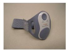
Fig. 2. BodyMedia SenseWear Pro2 Armband for measurement of GSR and skin temperature
